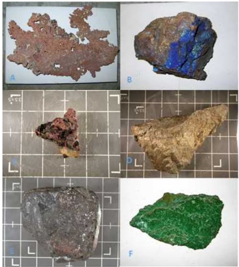
Figure 2: The different forms of copper. A) Native copper; B) Azurite; C) Cuprite; D) Chalcopyrite; E) Chalcocite; and F) Malachite. Photo Credit: Arizona Geological Survey.
