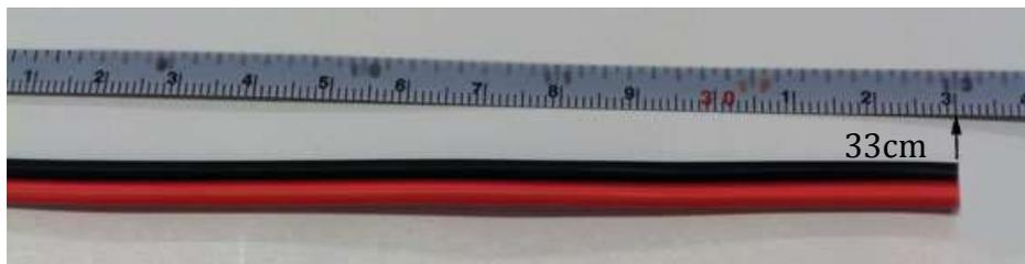
Figure 2. 33 cm length of 18-gauge copper wire.
