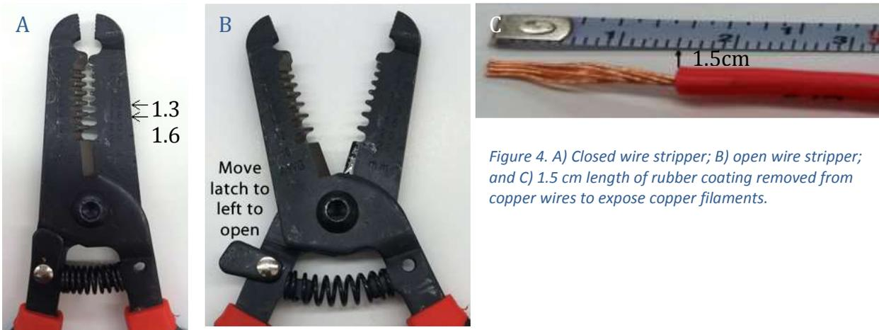
Figure 4. A) Closed wire stripper; B) open wire stripper; and C) 1.5 cm length of rubber coating removed from copper wires to expose copper filaments.
