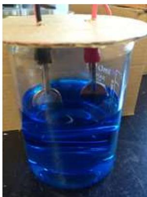
Figure 8. Electrodes immersed in the electrolyte solution.
