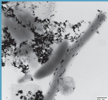
Elemental tellurium nanoparticles (black flakes) attached to microorganisms taken using transmission electron microscopy (Photo credit: Dr. Reyes Sierra and Tony Day).
